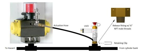
Install the Selector Valve assembly and a tee for the UVO / Release fitting approx. 1.0 feet apart in the fire suppression agent piping network.
